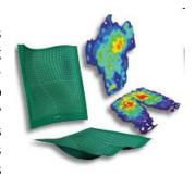
for measuring body-seat pressure, such as those used for seating optimization in the automotive sector.
